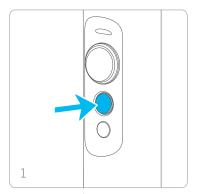
Click the function button five times. The motors will stop working. Status indicator turns solid blue
